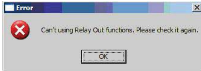
(4) If another user is already using Relay Out, the following message will be displayed when the Start button is pressed. Relay Out may be used when that user is done
