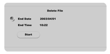
To delete a specific file range from the current recording HDD. This menu does not affect backup disk. The beginning of the range is always the beginning of the recording on the HDD.
