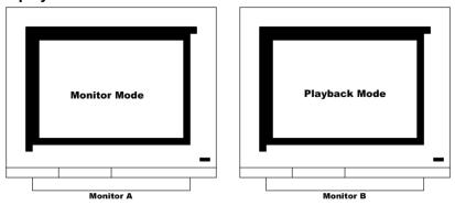
Administrator can monitor multi-cannnels by split screen mode in Monitor A, and search/playback 1 channel by single full screen in Monitor B simultaneously.
