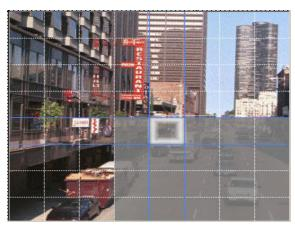
Press the "Custom Area" button, to customize the motion detection area. The area is divided into 64 blocks (8 x 8).
